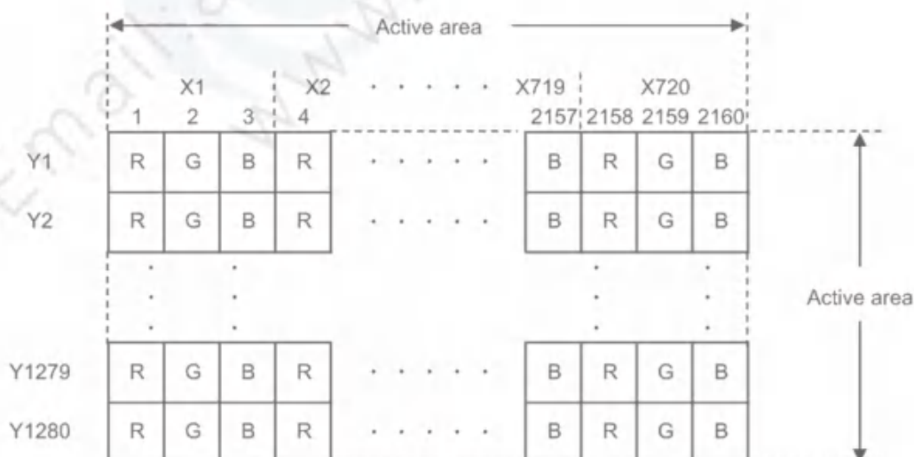
Dot arrangement (FPC cable placed low)
