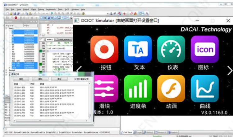
Figure 12-3 Keil development environment and virtual serial screen binding debugging
