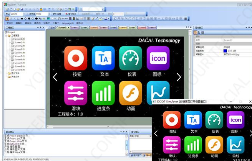
Figure 12-1 Main interface of VisualTFT
