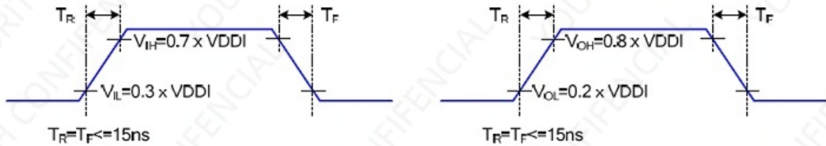
Figure 2 Rising And Falling Timing for Input And Output Signal
