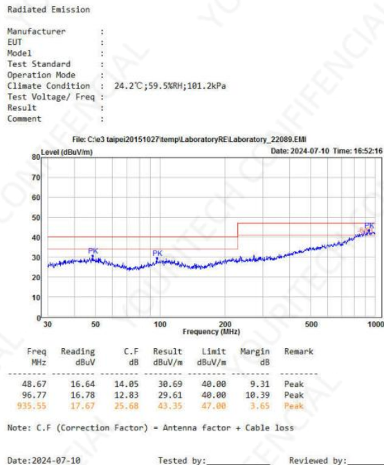
Figure 5-6: Horizontal direction of radiation measurement
