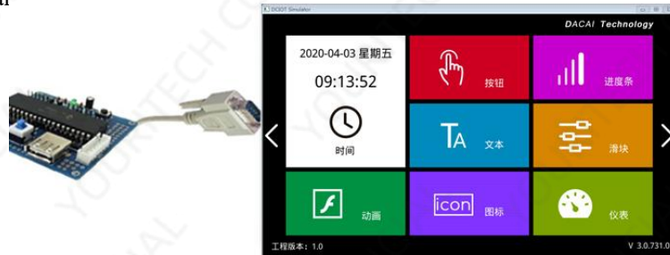
Figure 6-2 The serial port of the user's single-chip microcomputer is debugged online with the "virtual serial port screen".
