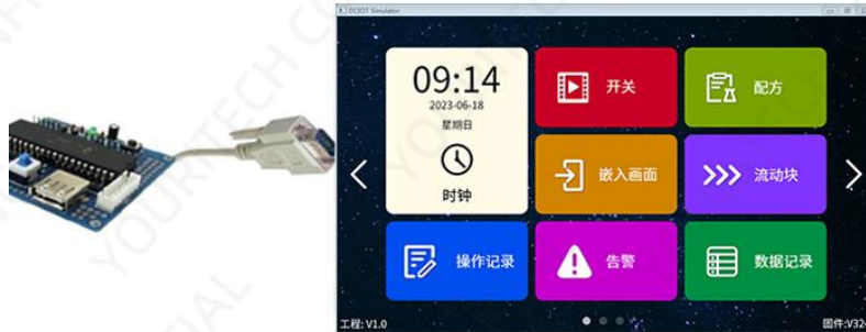
Figure 7-2 Online debugging between the serial port of the user's single-chip microcomputer and the HMI simulator
