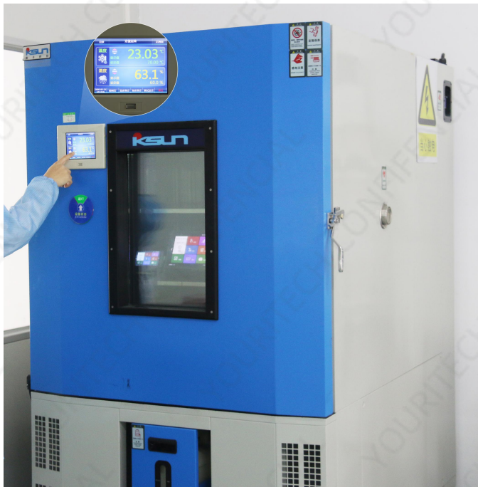
Figure 6-3 High and low temperature aging test
