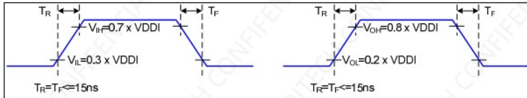
Figure 2 Rising and Falling Timing for I/O Signal
