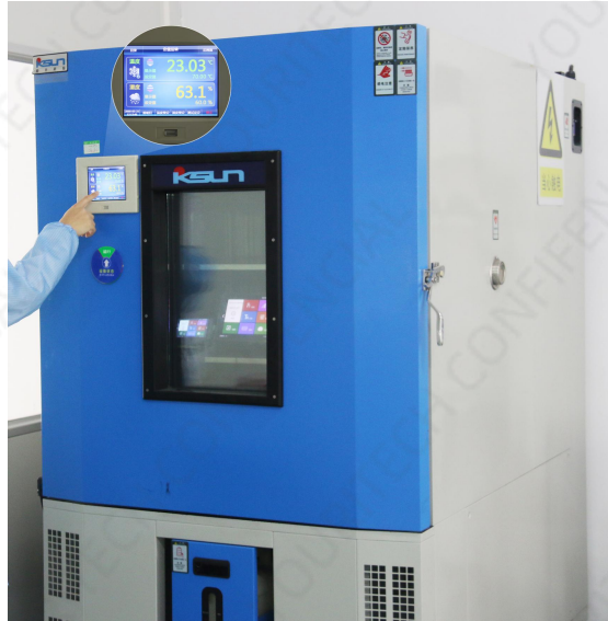
Figure 6-3 High and low temperature aging test diagram
