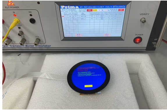
Figure 6-4 Group pulse test diagram
