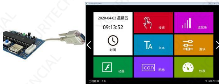
Figure 13-2 Online debugging of the serial port of the user single-chip microcomputer and the "virtual TFT simulation"
