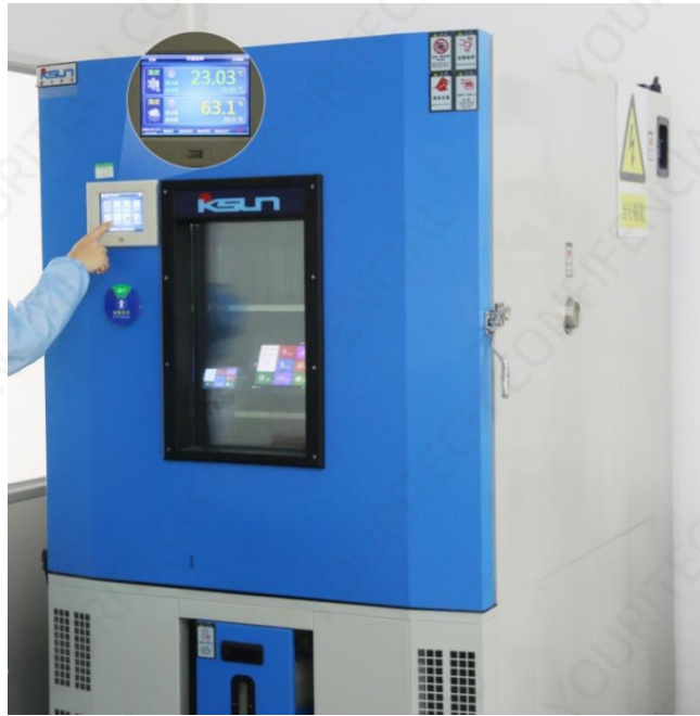
Figure 3-3 High and low temperature aging test diagram
