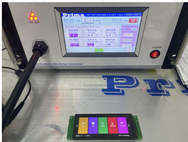
Figure 5-2 ESD test diagram
