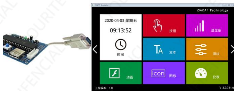
Figure 11-2 Online debugging of the serial port of the user single-chip microcomputer and the "virtual TFT simulation"
