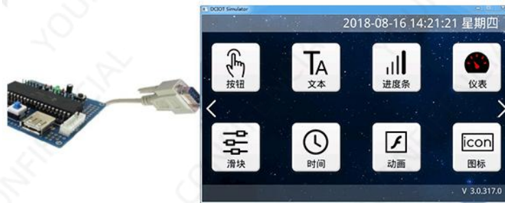
Figure 10-2 Online debugging of the serial port of the user single-chip microcomputer and the "virtual TFT simulation"
