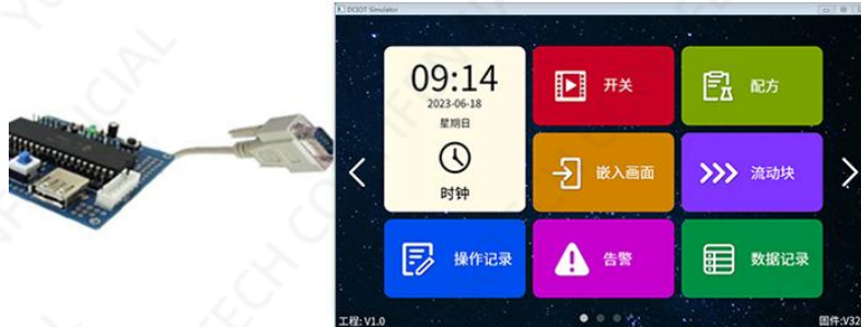
Figure 7-2 The serial port of the user's single-chip microcomputer is debugged online with the "HMI simulator"
