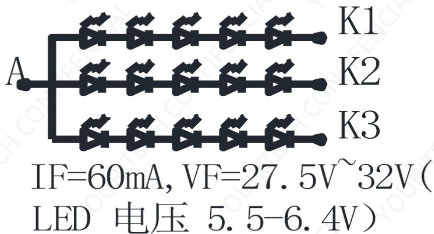
Fig. 3-1 LED test circuit diagram
