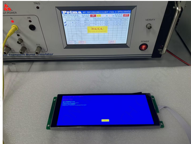
Figure 5-4 group pulse test diagram
