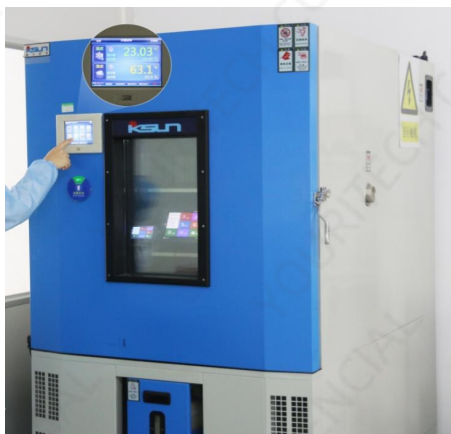
Figure 5-3 High and low temperature aging test diagram
