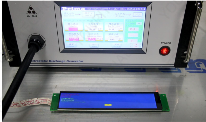
Figure 5-2 ESD test diagram
