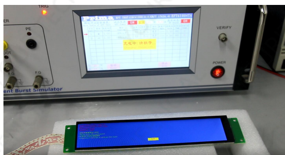
Figure 5-4 Group pulse test diagram
