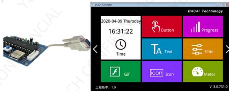
Diagram 9-2 Online debugging of serial port of user's single-chip microcomputer and virtual serial port screen
