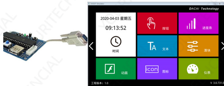
Figure 10-2 Online debugging of the serial port of the user single-chip microcomputer and the "virtual TFT simulation"
