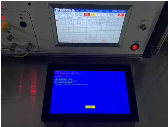
Figure 5-4 Group pulse test diagram
