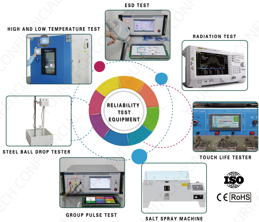
Figure 5-1 Reliability Test Equipment
