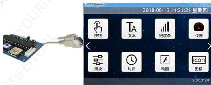
Figure 8 -2 Online debugging of the serial port of the user single-chip microcomputer and the "virtual TFT simulation"
