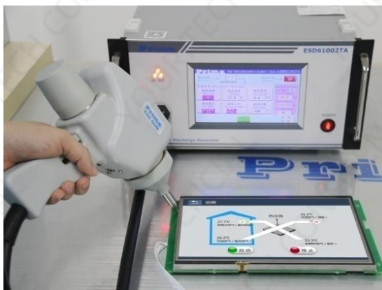
Figure 3-2 ESD test diagram
