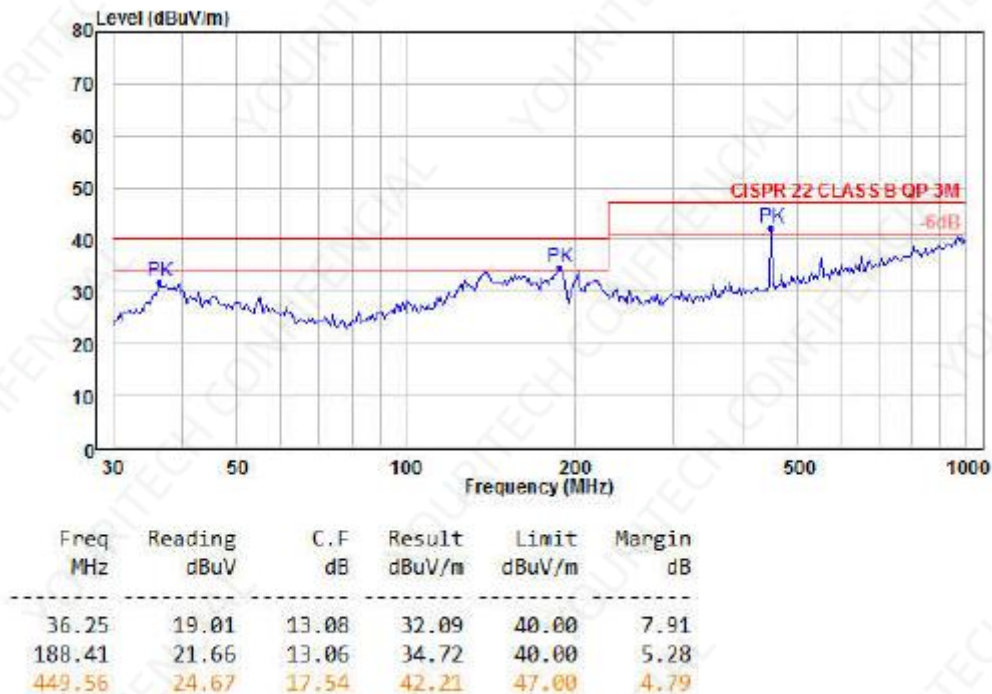
Figure 3-7: Radiation test vertical
