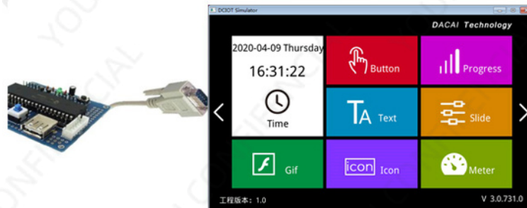
Diagram 10-2 Online debugging of serial port of user's single-chip microcomputer and virtual serial port screen
