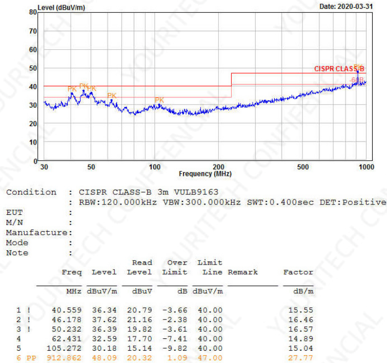
Diagram 3-7 Vertical direction of radiation test
