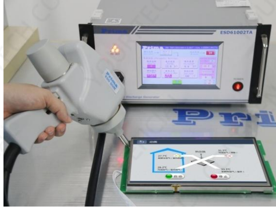
Figure 5-2 ESD test diagram
