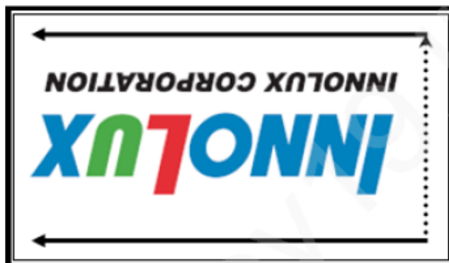
Fig. 2 Reverse scan (PCBA on the bottom side) ( pin 17, REV_SCAN = High_3.3V )
