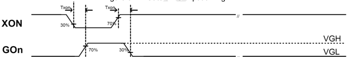
Figure 5.2.2 Gate driver input timing (continued)
